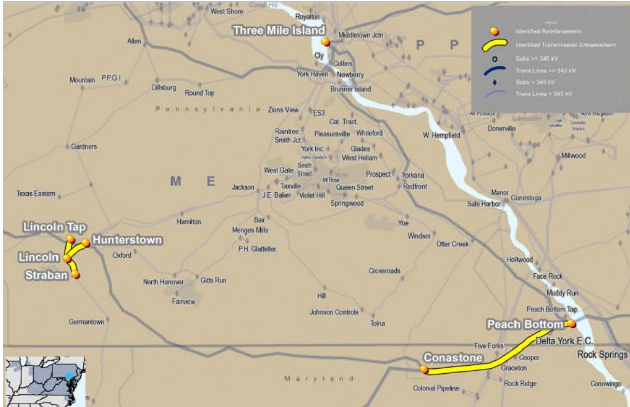
Map No. 1: n-1 Single Contingency Reliability Criteria Violations – September 2018 Analysis without Project 9A (2023 Study Year)
