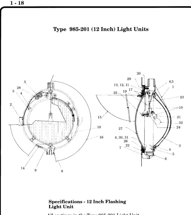
All castings in the Type 985-201 Light Unit are aluminum, with sheet aluminum hood and background.
