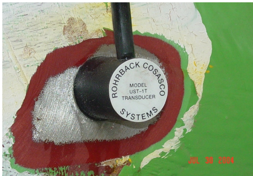
Figure 3: UT Probe Installation on the Ontario Drip
