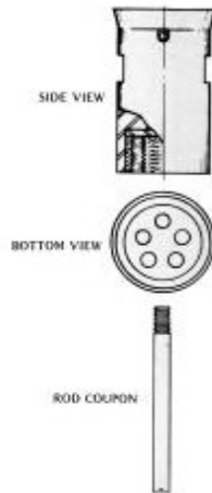
Figure 3 – Multiple Rod Coupon Assembly
