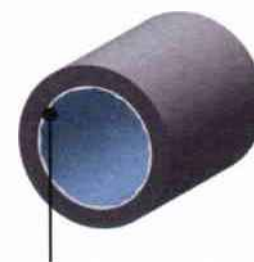
A protective layer of Orthophosphate forms to prevent pipe corrosion.
