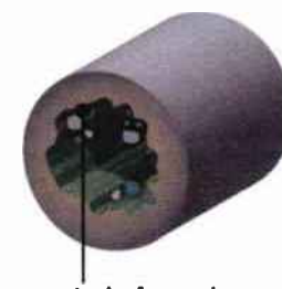
Lack of corrosion control allows lead to leach from pipes into water.
