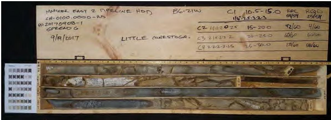
Photograph 1: B6-21W, Samples C-1 to C-4 (10.5 to 30 feet)
