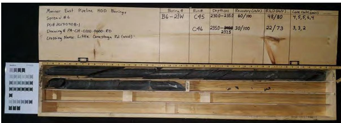
Photograph 12: B6-21W, Samples C-45 to C-46 (230 to 237.5 feet)
