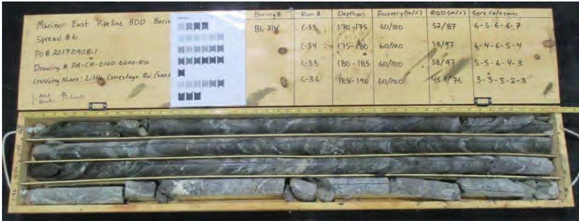
Photograph 9: B6-21W, Samples C-33 to C-36 (170 to 190 feet)
