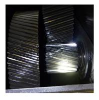
Real picture of the 3 gear-reduction gearbox shown in the diagram on the left. Not all gears are visible in this picture. Gear oil is an oil bath and splash lubrication system.
