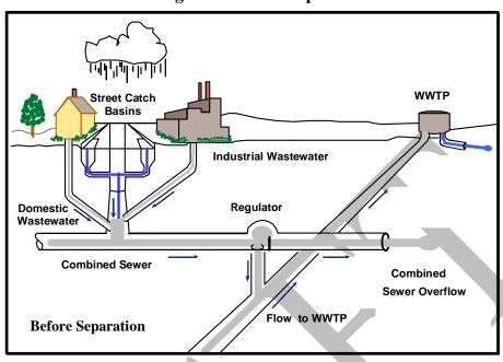
Figure 1. Sewer Separation
