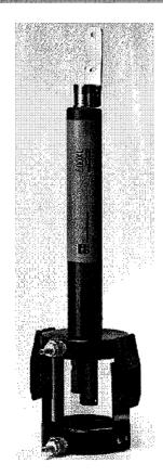
YSI Model 5083 flow cell and 600XL. This is an ideal combination for groundwater applications.
