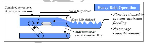
Existing, unused conduit storage involves using existing pipes that have been taken out of service for various reasons and re-introducing them as a form of storage. As discussed earlier under regulator optimization, making modifications to fixed weir regulators (static controls) within existing conduits can re-direct flows into nearby abandoned pipes, resulting in additional storage upstream of the regulator structure and a reduction of overflows during small wet weather events. However, the
