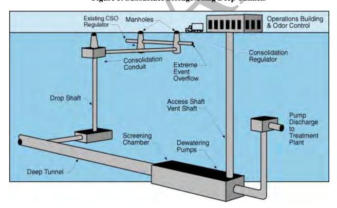
Figure 3. Subsurface Storage Using Deep Tunnels
