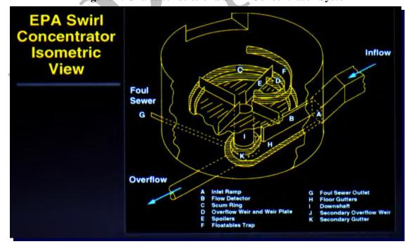
Figure 4. Characteristics of a Swirl Concentrator System
